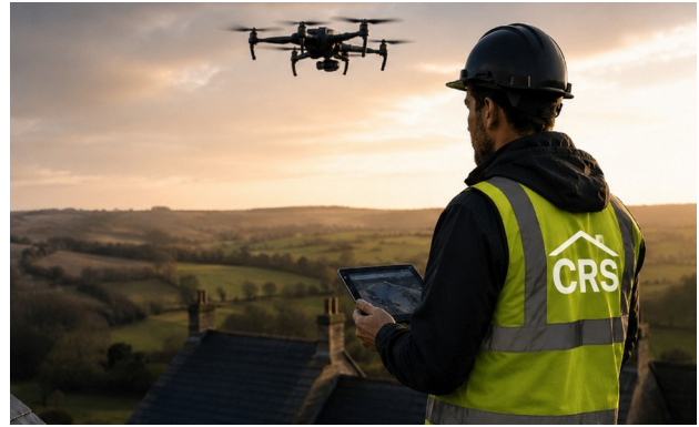
Aerial inspection supports safe evidence gathering while keeping operatives off fragile roof areas.
